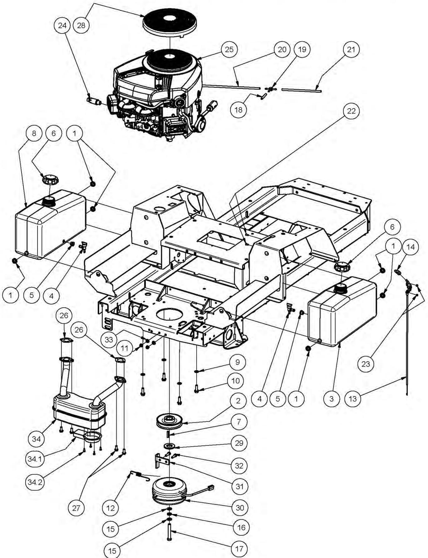
**ENGINE AUXILLARY COMPONENTS 24HP B&S 48" Cut Only**
